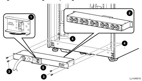
Figure 2-7 Removing and Replacing the Power Distribution Unit
